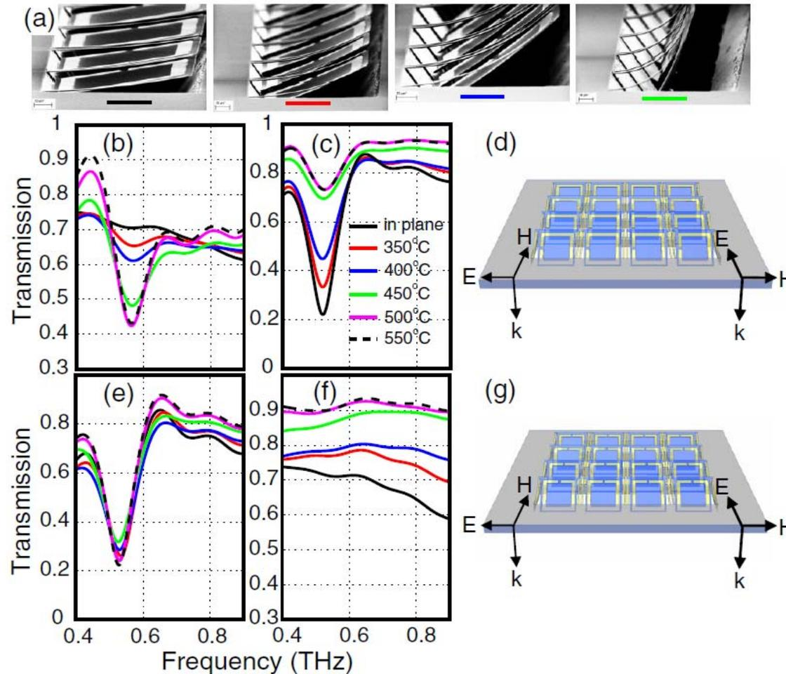
Reconfigurable Terahertz Metamaterials, Hu Tao, A.C. Strikwerda, K. Fan, W. J. Padilla, X. Zhang, and R. D. Averitt, PRL 103, 147401 (2009)
