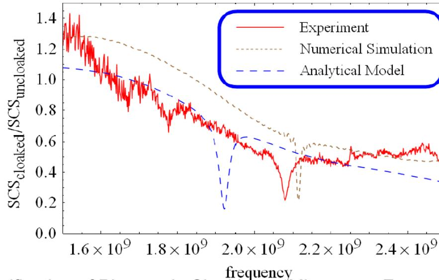
Experimental Verification of Plasmonic Cloaking at Microwave Frequencies with Metamaterials
