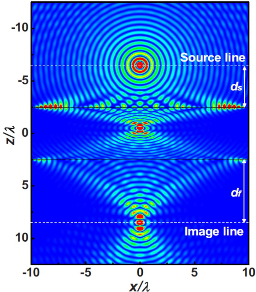
Anisotropic metamaterial lens, with parameters  $\epsilon_x = \mu_y = -2 + 0.001i$  and  $\mu_z = -0.5 + 0.001i$
