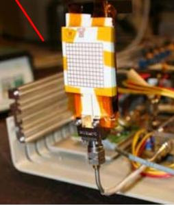
Actual 1.25 Gigabit/s Ethernet data was transmitted wirelessly between two computers using this high gain antenna structure
