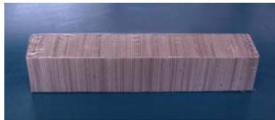
Complete NIM slab ( ~ 900 Unit Cells )
