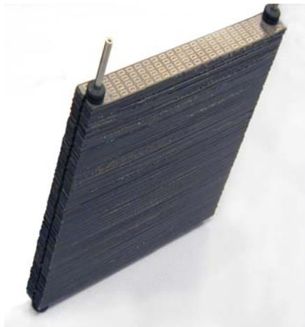
➤ “Precisely cut, aligned” and assembled of 161 strips
